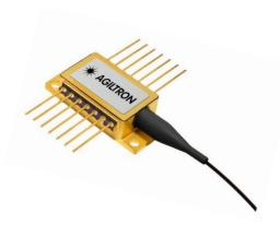
The 1064nm series laser diodes are fabricated in a hermetically sealed 14-pin butterfly package. The laser diodes contain a monitor photodiode, thermoelectric cooler (TEC), and a thermistor to secure high-quality laser performance. Our laser products are Telcordia GR-468 qualified and in compliance with RoHS Directives.
